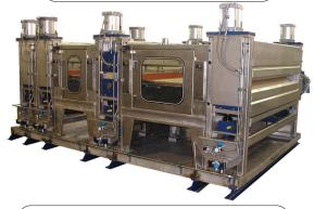
A method to remove rolling oil from metal strip using water at high temperature and pressure.
