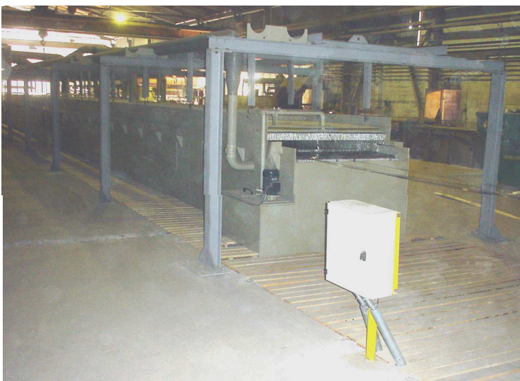
CONTINUOUS PICKLING UNIT - 40 STRANDS "TYPE CLOSED"
